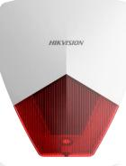
The wired sounder is used to connect to wired control panel, by using 12v outpout voltage from panel, the sounder can alarm up to 105dB sound. The sounder can be used both internal or external, the LED fash and the sounder indication can be configured separately.
