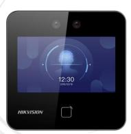
Face recognition terminal adopts deep learning algorithm, which helps to recognize the face faster with higher accuracy. It also supports multiple authentication modes: face/card authentication, etc. It can be applied in multiple scenarios, such as buildings, enterprises, financial industries, and other important areas.
